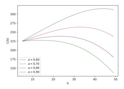
**Fig. 9.** The reward function C(b) defined by Eq. (9) and to be maximized; b is the energy level switching the performance of UAV from normal mode to energy saving mode, for linear function  $\Theta$  defining the decrease with time of the value of previously gathered data, see Eq. (11), with parameters  $\mu_2 = 0.10$ ,  $a \in [0.6, 0.9]$ .
