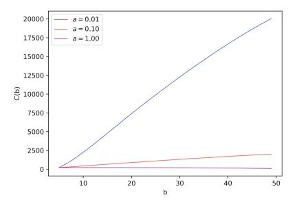
**Fig. 8.** The reward function C(b) defined by Eq. (9) and to be maximized; b is the energy level switching the performance of UAV from normal mode to energy saving mode, for linear function  $\Theta$  defining the decrease with time of the value of previously gathered data, see Eq. (11), with parameters  $\mu_2 = 0.10$ , a = 0.01, 0.1, 1000
