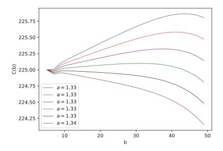
**Fig. 6.** The reward function C(b) defined by Eq. (9) and to be maximized; b is the energy level switching the performance of UAV from normal mode to energy saving mode, for exponential function  $\Theta$  defining the decrease with time of the value of previously gathered data, see Eq. (10), with parameters  $\mu_2 = 0.15$ ,  $a \in [1.326, 1.336]$
