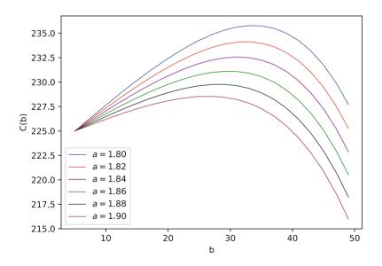
**Fig. 3.** The reward function C(b) defined by Eq. (9) and to be maximized; b is the energy level switching the performance of UAV from normal mode to energy saving mode, for exponential function  $\Theta$  defining the decrease with time of the value of previously gathered data, see Eq. (10), with parameters  $\mu_2 = 0.1$ ,  $a \in [1.8, 1.9]$
