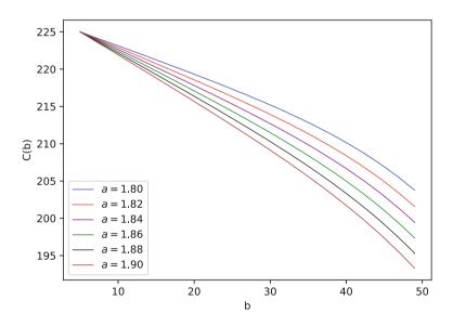
**Fig. 5.** The reward function C(b) defined by Eq. (9) and to be maximized; b is the energy level switching the performance of UAV from normal mode to energy saving mode, for exponential function  $\Theta$  defining the decrease with time of the value of previously gathered data, see Eq. (10), with parameters  $\mu_2 = 0.12$ ,  $a \in [1.8, 1.9]$
