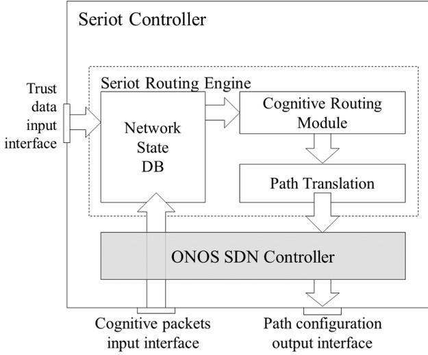
Fig. 6. SRE: The SerIoT Controller and Routing Engine.
