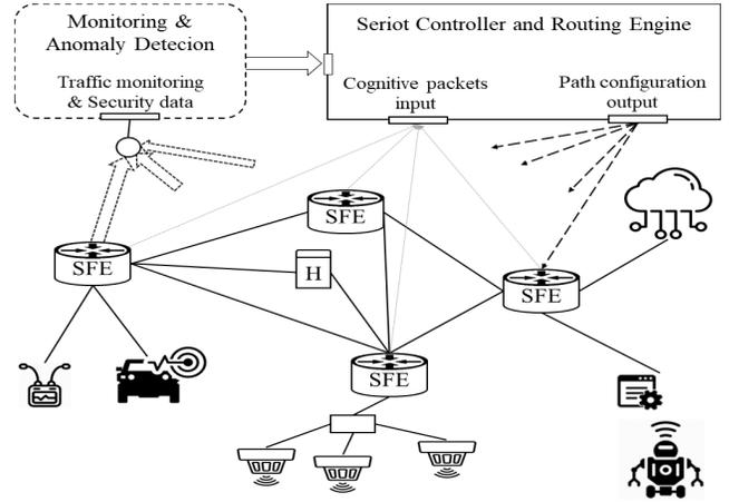
Fig. 4. Overview of the Secure IoT network System Architecture.
