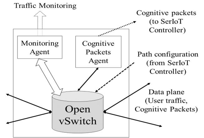
Fig. 5. SFE: the SerIoT Forwarding Element.
