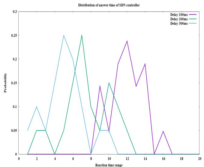
Fig. 10. Measured Probability Distribution of the Reaction Time of the system as a whole, including the network and the SRE, as viewed by the end user.
