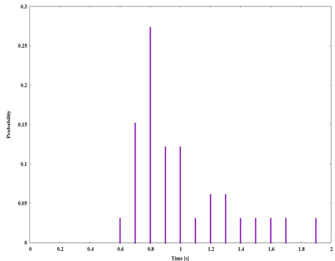
Fig. 13. Distribution of Routing Engine Reaction Time to a sudden substantial change in the Trust Metric  $T(.,.)$ .
