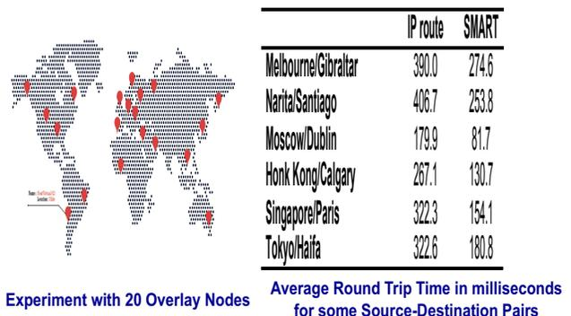
Fig. 3. Average Round-Trip Delay measured during a one week experiment that compared the use of the IP protocol with SMART for several intercontinentally distributed overlay nodes. The data shows a distinct reduction of delay when SMART is used.
