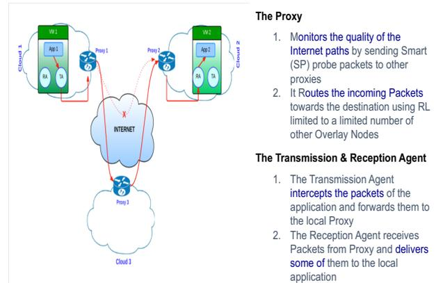
Fig. 2. The software architecture of the SMART overlay node.
