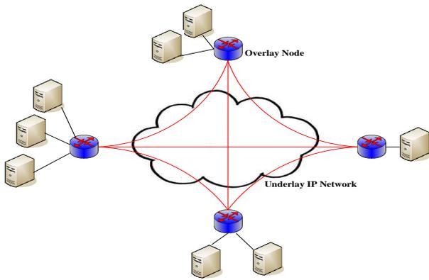
Fig. 1. Schematic Representatin of an Overlay Network.
