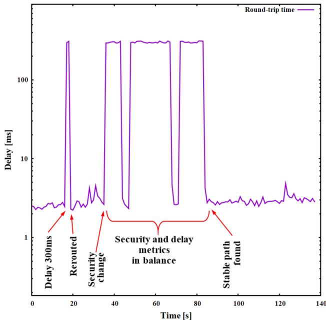
Fig. 14. System reactions to changes in delay and security. Note that the  $x$ -axis describes the course of real events in seconds, while the  $y$ -axis plots the reaction times of the system as a whole, in milliseconds, to the events that occur along the  $x$ -axis.
