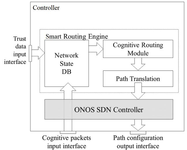
Fig. 8. The Smart Routing Engine SRE acting as an SDN Controller that takes decisions for Goal Based Routing using the RNN and RL.
