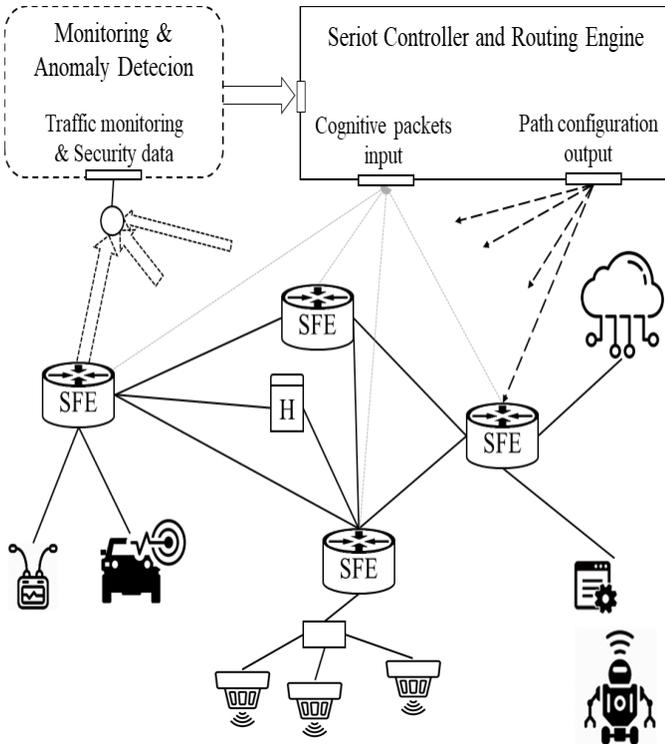
Fig. 7. Overview of the networked architecture.
