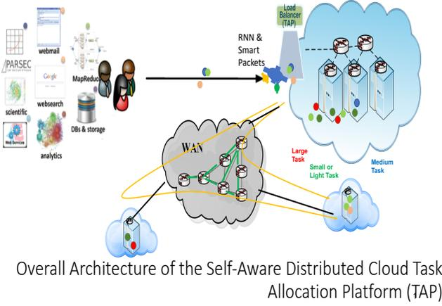
Fig. 4. Overall architecture and operation of the Task Allocation Platform which distributes tasks locally to a Cloud server, or distributes jobs remotely via the Internet to other Fog and Edge servers. On the tight-hand-side of the figure we see that tasks may be of different types and may have wide ranging requirements in terms of memory occupancy and task execution time, while their QoS requirements may also vary widely.
