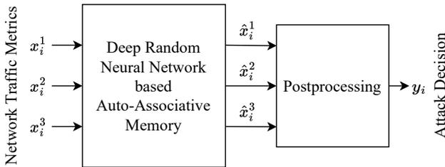
Fig. 2. The structure of the IDS system that computes the decision variable  $y_i$  from the network traffic metrics  $[x_i^1, x_i^2, x_i^3]$  with the DRNN based Auto-Associative Random Neural Network (AAD RNN) and the postprocessing module.
