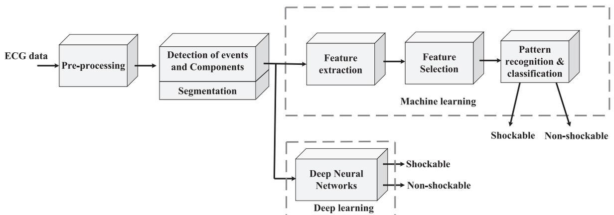
Fig. 5. General block diagram of a CAAC system.
