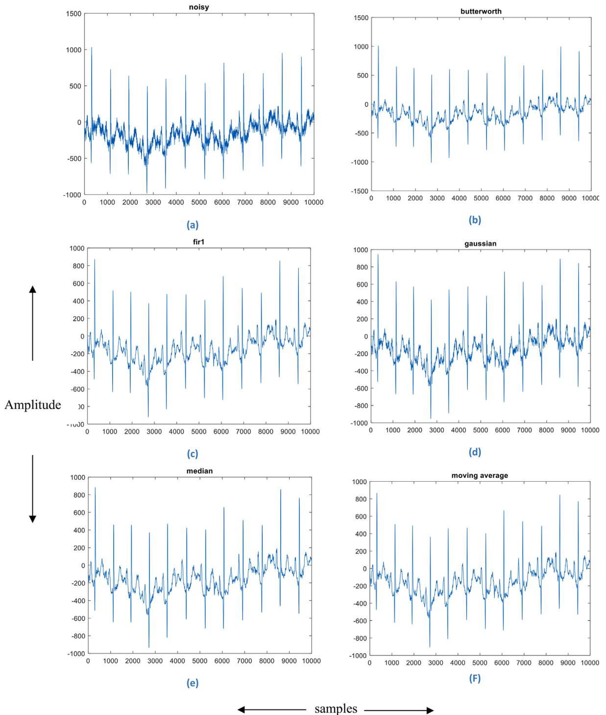
**Fig. 6.** Effect of using several filtering techniques: a) the noisy signals, b) after applying Butterworth filtering, c) finite impulse response (FIR) filter, d) Gaussian filter, e) Median filter, f) moving average filter.
