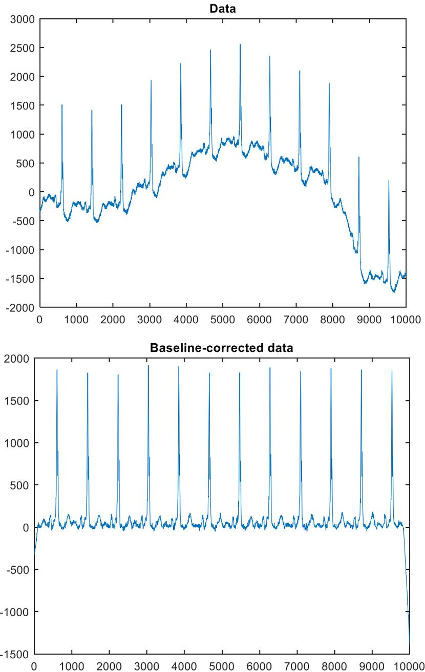
Fig. 7. Elimination of baseline wander using filtering methods.
